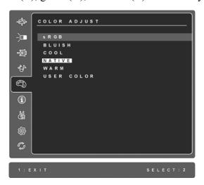
**sRGB-**This is quickly becoming the industry standard for color management, with support being included in many of the latest applications. Enabling this setting allows the LCD display to more accurately display colors the way they were originally intended. Enabling the sRGB setting will cause the Contrast and Brightness adjustments to be disabled.
