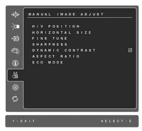
**H./V. Position (Horizontal/Vertical Position)** moves the screen image left or right and up or down.
